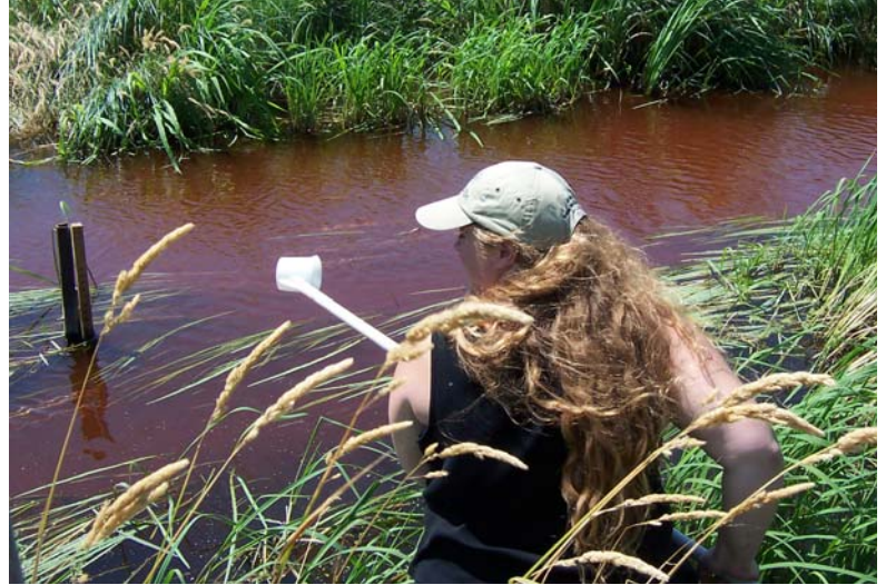
Brandy Elf conducting a water "time of travel" study using an inert dye which is put upstream of the wetland and then measured downstream in timed increments as the dyed water flows through the wetland.
